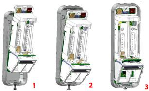
Figure 5 – Attaching the Main Unit
